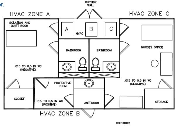
Note: Systems A, B, and C are the Dedicated "Isolation Mode "systems, each system is individually operated and controlled. The Supplementary HVAC systems for "Normal mode" are not shown.
